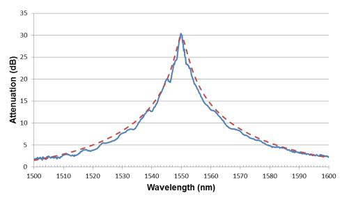
Wavelength response of  $LP_{\sigma 1}$  transmission for mechanical LPG. Solid curve shows experimental results and dashed curve theoretical curve with the same number of coupling points and coupling coefficient.
