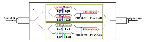
Figure 5. DP QPSK modulator numbering for D0158 MBC
