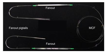
Fanouts are typically shipped in spliced pairs, as shown here for a 7-core MCF. This configuration enables full testing of insertion loss and crosstalk for each pair. MCF and pigtail lengths can be tailored to your needs. Fanout pigtails, two pairs of 7 fibers shown on left in this example, are typically standard singlemode fibers.
