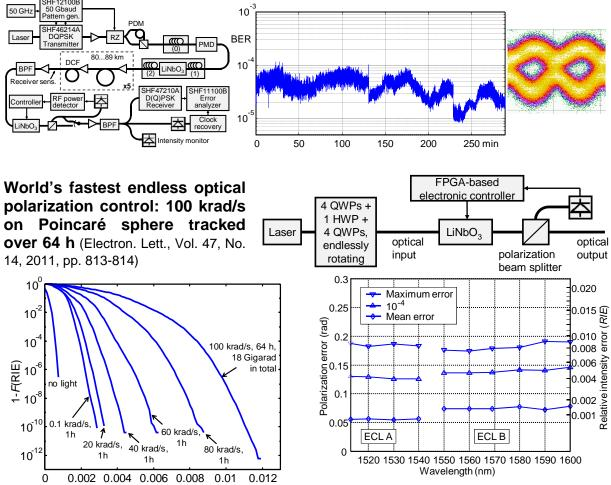
Complementary distribution function 1-F(R|E) of relative intensity error (R|E) for 1 hour at 0.1, 20, 40, 60, 80 krad/s, and for 64 hours at 100 krad/s scrambling speed (18 Gigarad in total). The zero point (R|E=0) is determined without light.
