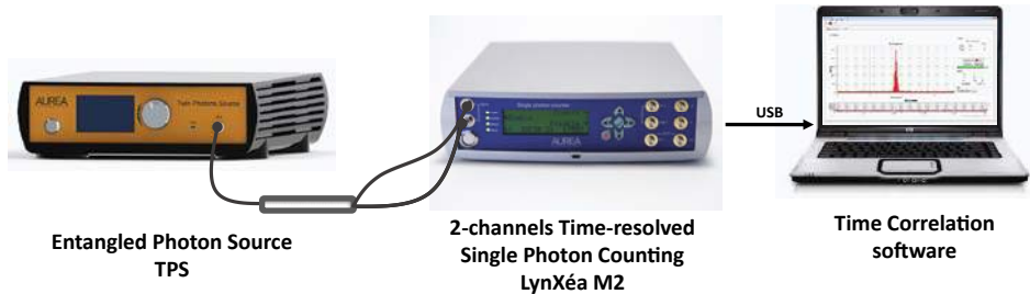
Photon pair correlation measurement
