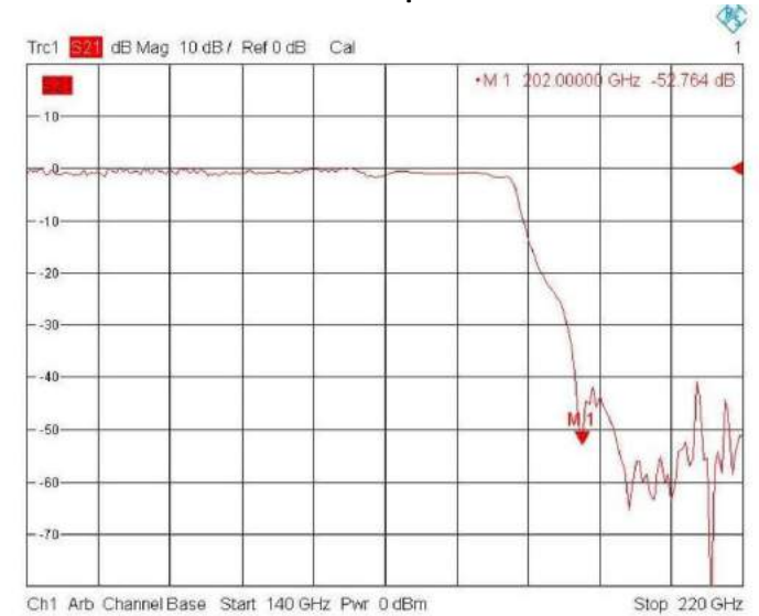
Model VTBPF-06 Band Stop Filter 200 – 220 GHz
